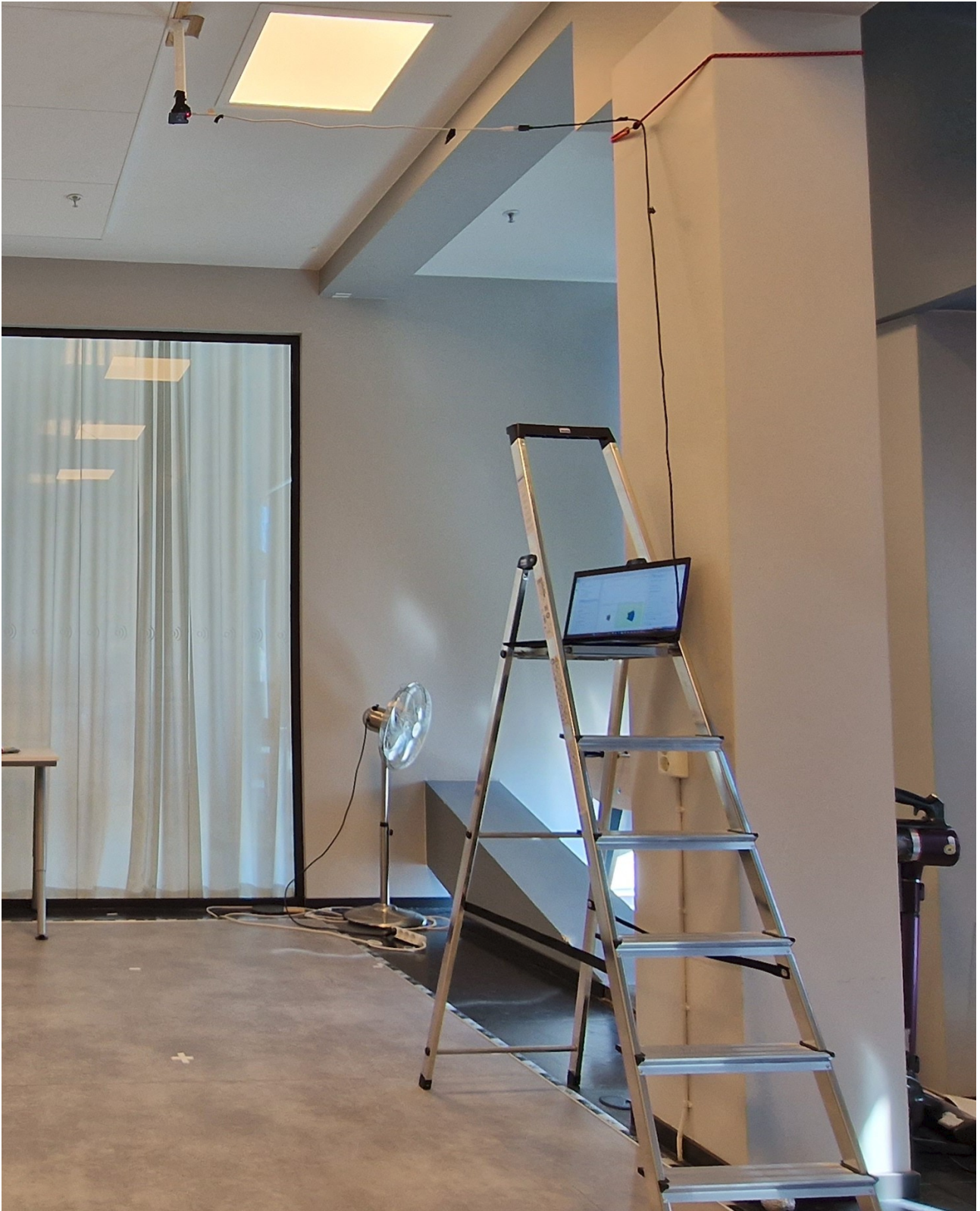
Figure 2: Sensor mounted on the ceiling about 3 m up from the floor. Setup used for test cases 7 and 8.
