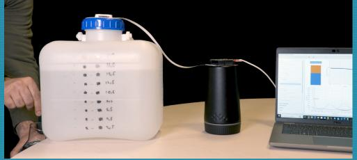
In the example above we are slowly emptying our small test tank and millimeter accuracy is achieved throughout the whole range. Try it for yourself with Acconeer's Exploration Tool. Proof of concept for tank level use case
