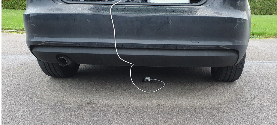
Figure 4: Sensor under the tank
