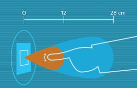
In the tests, we used far and short range simultaneously. We first registered a button press at long range (blue) and then another one at short range (orange). The bottom graph shows the number of detections above the threshold.
