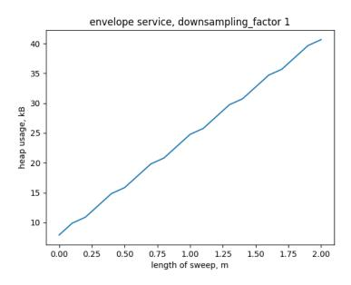
The figure above gives an indication of how much memory that is allocated on the heap in relation to sweep length and acc\_service\_envelope\_get\_next() is used to retrieve the data.
