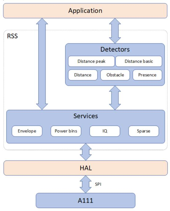
Acconeer also provides several easy to use detectors that are implemented on top of the basic data services. The detectors provide an interface for higher level tasks like distance measurements, motion detection etc.
