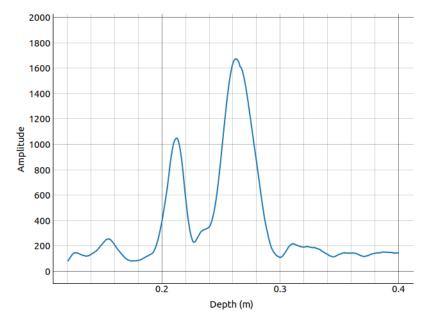
When a profile is choosen to improve radar loop gain, the radar sends out more energy, and the receiver has a higher gain setting which leads to a higher amplitude in the received signal. The internal filter parameters are also different which gives a smoother signal where noise and fine details have been removed. The graph below shows the same two objects as before but with profile 2 enabled.
