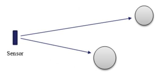
Assume that you have a setup with two objects like in the figure above. When plotting the Envelope data recorded using profile 1, which is optimized for maximum depth resolution, you will get a graph similar to the one below.
