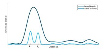
The figure above shows the envelope signal of the same objects with two different profiles, one with a short pulse and one with a long pulse.
