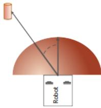
The distance is the actual distance of the obstacle to the radar sensor and the angle is the measured with respect to the direction of motion of the radar sensor. If you need the "normal" distance of the obstacle to the sensor, you can calculate it via the relation cos(alpha)d.
