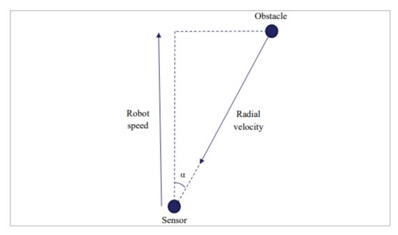
Radial velocity is used to estimate the angle of an obstacle using
