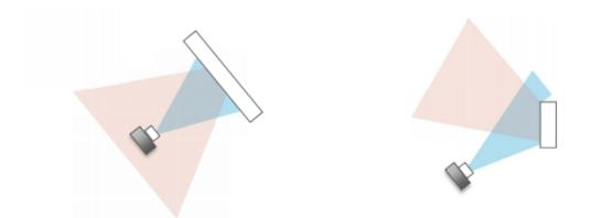
Figure above show object with normal incidence resulting in good reflectivity and object with oblique incidence resulting in reduced detectability
