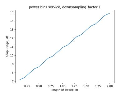
The figure above gives an indication of how much memory that is allocated on the heap in relation to sweep length and acc\_service\_power\_bins\_get\_next() is used to retrieve the data.
