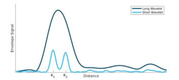
The figure above shows the envelope signal of the same objects with two different profiles, one with a short pulse and one with a long pulse.
