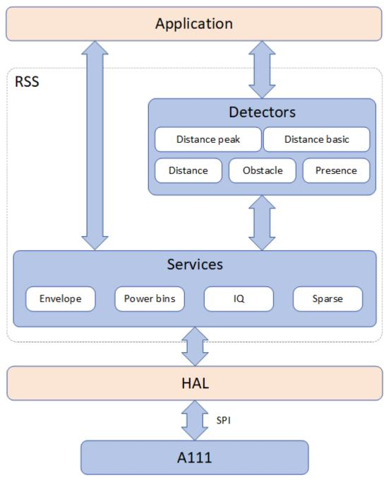
The detector is designed to detect movement with a low update rate to enable low power use cases as well as higher update rate to keep track of a person walking within the range of the sensor. The detector provides output data to detect movement as well as distance to where the movement occurred. This enable applications to implement smart presence algorithms and react on movement in different areas.
