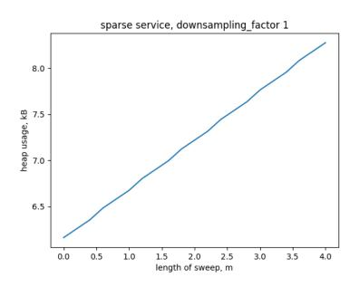
The figure above gives an indication of how much memory that is allocated on the heap in relation to sweep length and acc\_service\_sparse\_get\_next() is used to retrieve the data.
