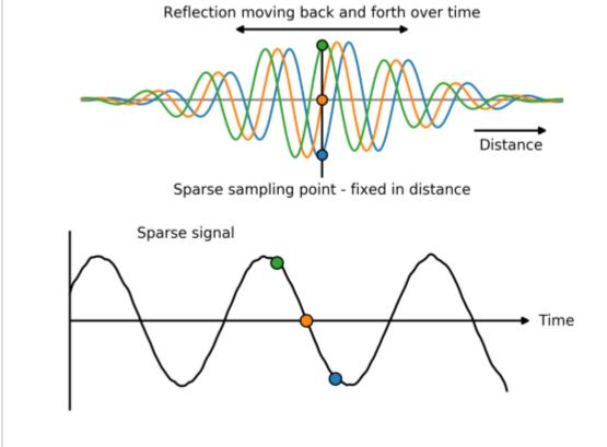
The above image illustrates how a single sparse point samples a reflected pulse from a moving target. Due to the movements of the target, the signal from the Sparse service varies over time. If the object is static, the signal too will be static, but not necessarily zero.
