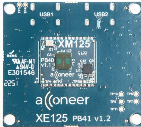
Picture 1. The XE125 top side where XM125 is mounted.
