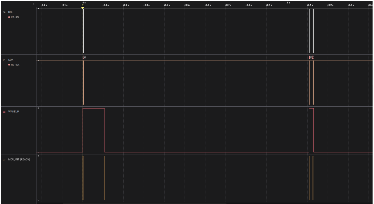
Low Power Example: Wake up, Setup Distance Detector, Power down, Wait 1s, Wake up, Measure distance, Power down
